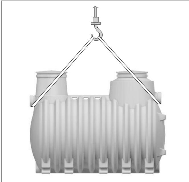
pect loads must be avoided. If a fork lift is used, the tanks must be secured while they are transported on the fork lift. It is not permissible to roll or drag the tanks across the floor. It is forbidden to roll or drag containers over sharp-edged surfaces. The containers used for loading and unloading may only be pushed or pulled on the loading platform of a lorry.
